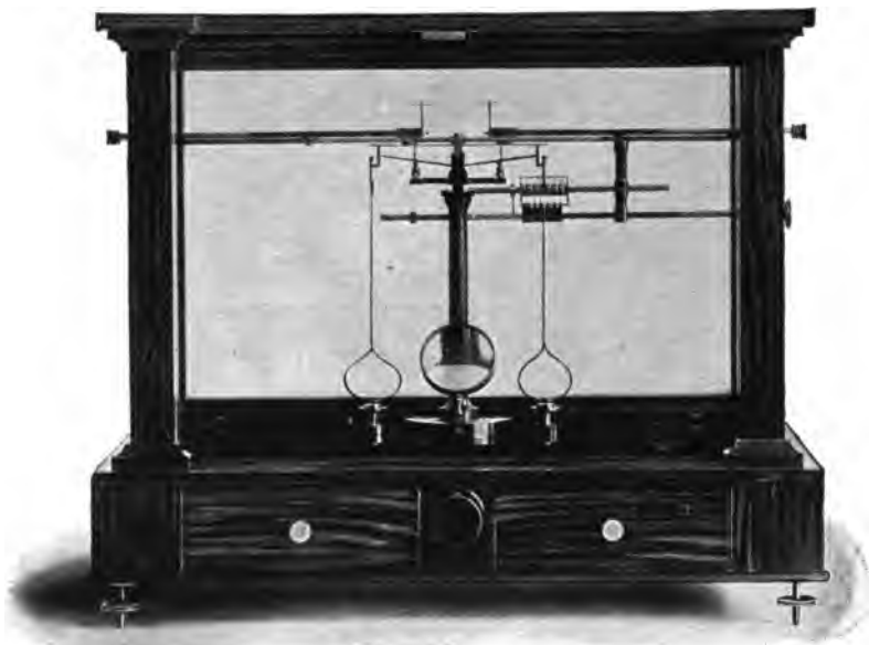
FIG. 41.—ASSAY BUTTON BALANCE.
